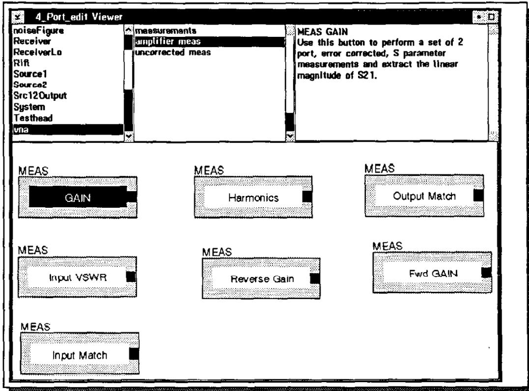
You create test plans, as previously shown, by copying buttons from other test plan panels (or from the Test Instrument Panels) and adding the buttons to a new test plan panel. For example to add the GAIN measurement button you select the **vna** instrument and the **amplifier meas** button types (shown above), select the **MEAS GAIN** button (highlight the button), and add the button to the test plan. The process takes just a few seconds. It is that simple and easy to create tests.
