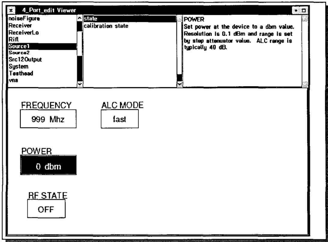
The Test System Viewer panels also provide the measurement state buttons. For example to select the source power state button in the previous example, you select the **Source1** instrument and the **state** button types (shown above), select the **POWER** state button (highlight the button), and add the button to the test plan.
