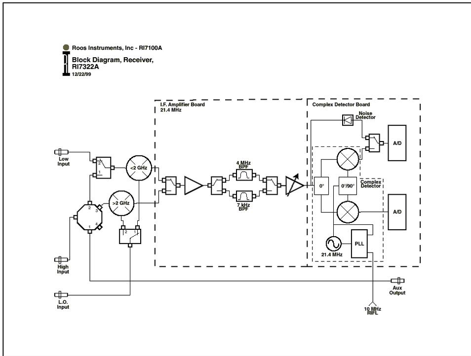
The microwave signals received by the System Receiver are down-converted to the 21.4 MHz IF frequency using the external Microwave System Local Oscillator (LO).
