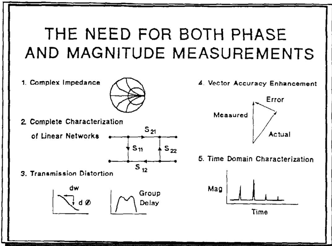
Before we discuss S parameters in detail, it may be useful to understand why we need to measure S parameters of an RF device and why phase information is useful. S parameter measurements (both amplitude and phase) are used to characterize the transfer characteristics (input to output response) of an RF device and to determine the complex impedance (both resistive and reactive components) of the device's RF inputs and outputs.
