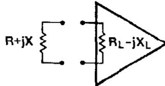
$P_{av} = kTB =$  Power Delivered to a Conjugate Load, i.e.  $R_L = R, X_L = X.$
