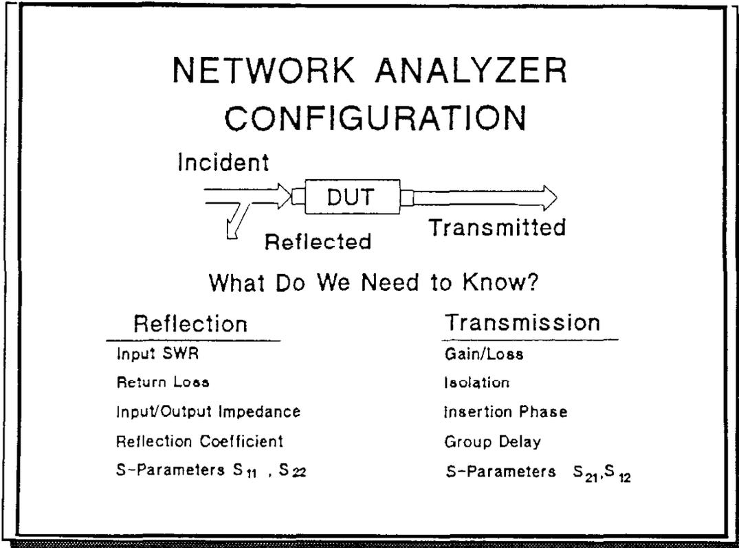
To fully analyze the magnitude and phase characteristics of a typical 2 port device (device with 2 RF connections), may require looking at the data in different ways. A vector network analyzer system provides you the flexibility to present the data in many different formats as shown in the slide.
