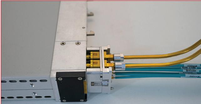
▲ Fig. 4 Modular blind-mate interface and fixture.
