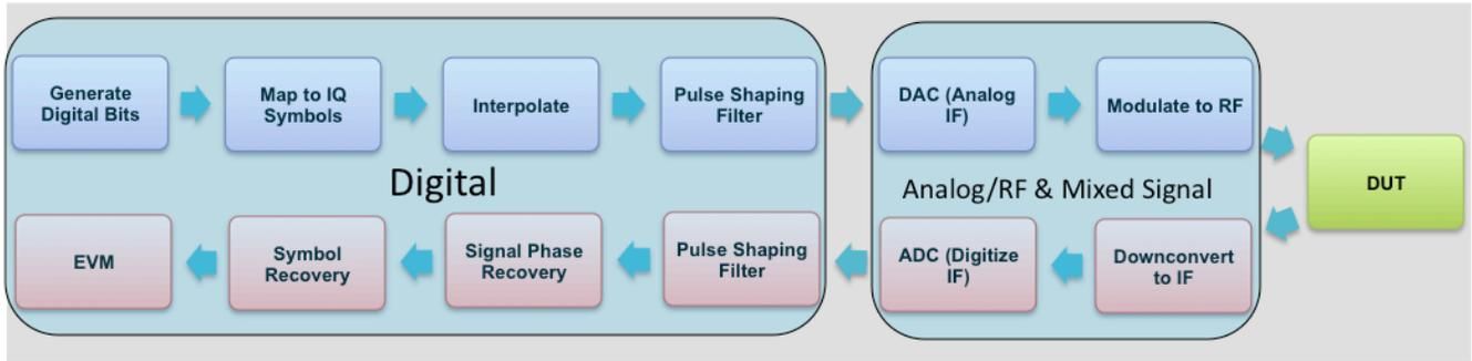
**Fig 1: Generic Flow Diagram for Measuring EVM from a DUT: Modulated Signal Generation (Blue/top path), Signal Demodulation and EVM (Red/Bottom Path). Each flow path is broken down into its' corresponding digital and RF/analog paths**
