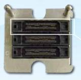
Digital Block: 40-pin, high-speed connector
